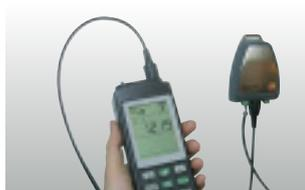
Inspection of transmitters with 4 to 20 mA interface
