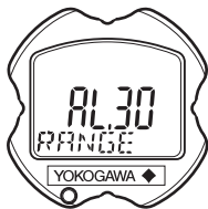
Self-diagnostic error on the integral indicator (Faulty transmitter)
