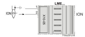
LME7 connection assignment: Terminal X10-05 pin 2 Flame signal ionization input
