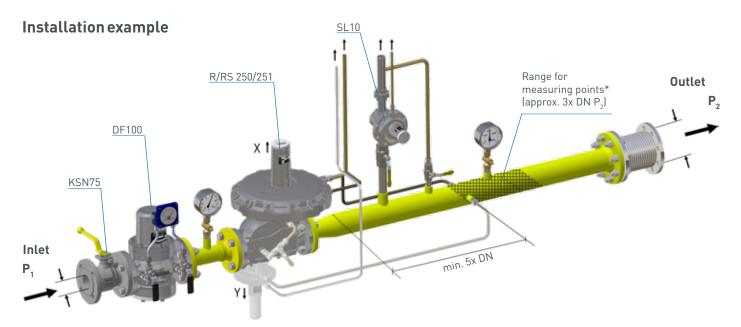
\*) Recommended max. velocity at the measurement line port 25 m/s
