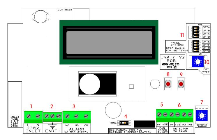
Power at 230 volts from a 3amp fused spur
